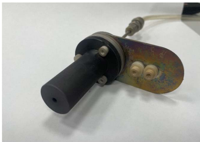
Figure 4. Photograph of heaterless hollow cathode after 25 h of operation.
